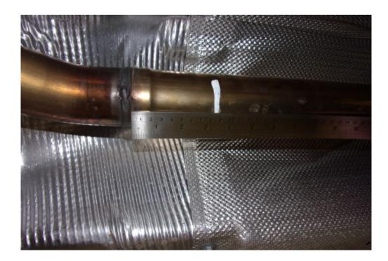
Cut the OE system 85mm in front of the weld (towards the front of the vehicle) and remove sharp edges
